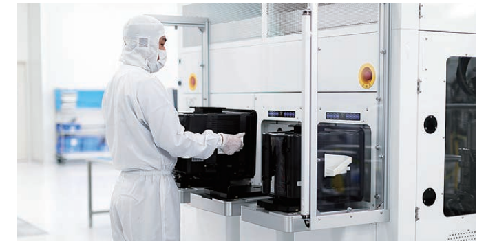
Canon ANELVA's sputtering equipment deposits uniform nanoscale film under vacuum
