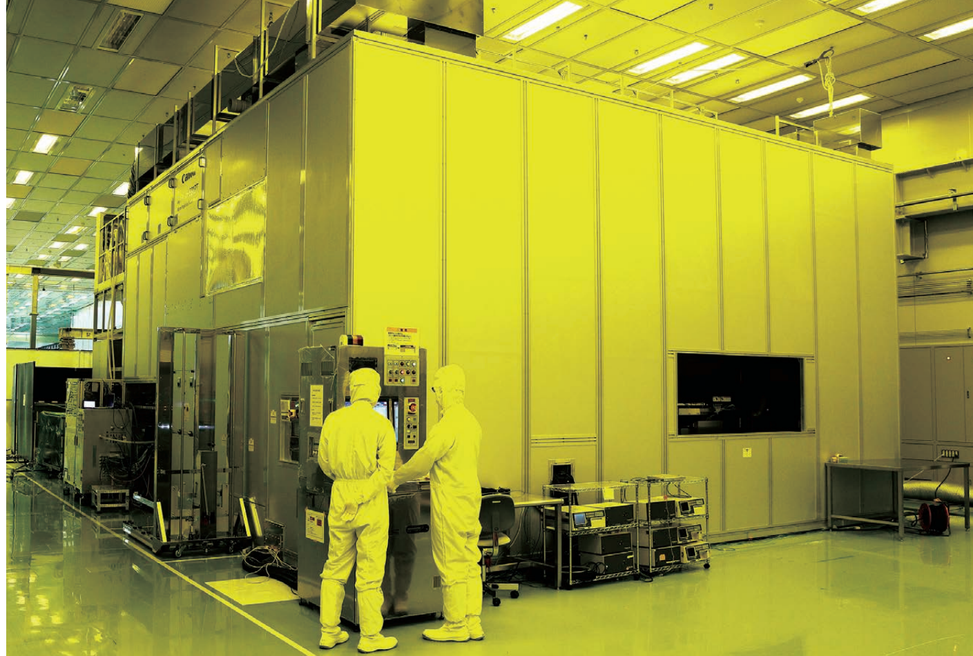
Canon Flat Panel Display (FPD) lithography equipment exposes circuit patterns on glass substrates
