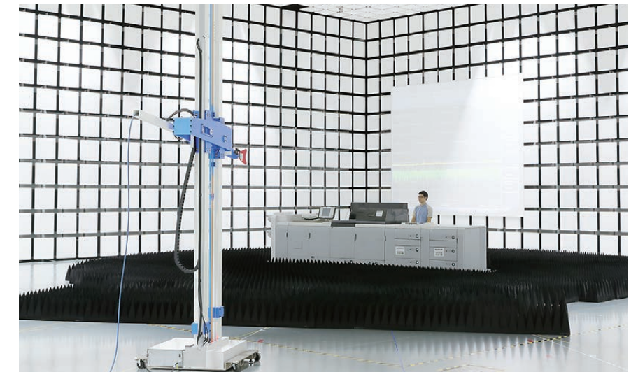
Canon's ISO/IEC 17025 certified anechoic chamber is qualified for third-party testing
