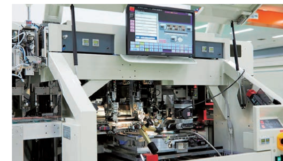
Canon Machinery's die bonder used to attach semiconductor chips
